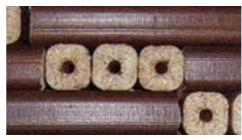
processes. The sawdust is compressed and the lignin contained in the wood can be softened, allowing it to act as a natural binder, producing a reformed log size product. Briquettes are dense and this reduces the amount of storage space required. They are clean to handle and easy to take home in 'ready to burn' retail packs.
