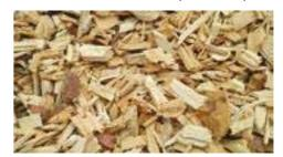
the appliance (especially domestic sized boilers) work at their optimum efficiency and reliability. Typical wood chip from a tree surgeon is too wet and variable in chip size for most appliances.
